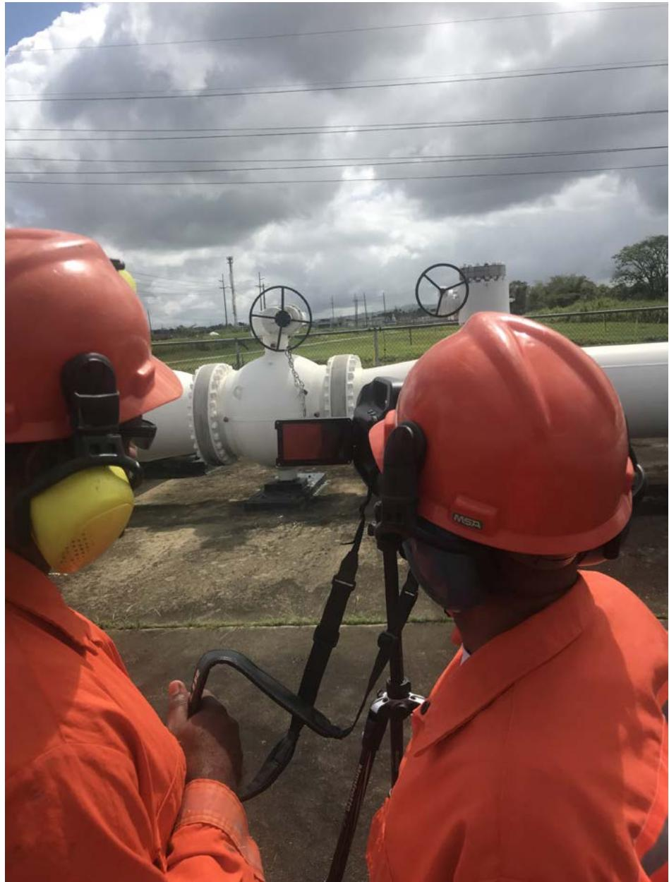
*An infrared camera is helping NGC visualise leaks along its lines*
